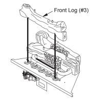
Figure 27 - Installing Front Log
